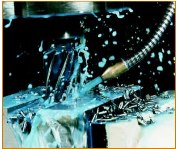
Effective heat removal yields good tool life and dimensional accuracy of parts.
